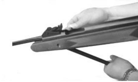
Fig.3 Once this has been done, then whilst holding the underlever down with one hand, insert a pellet in to the open breech.
