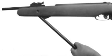
Fig.2 Hold the rifle handle by the stock with one hand whilst pulling down the underlever with the other. Pull this lever down fully until a “click” can be heard and the piston is then engaged on the trigger system.
