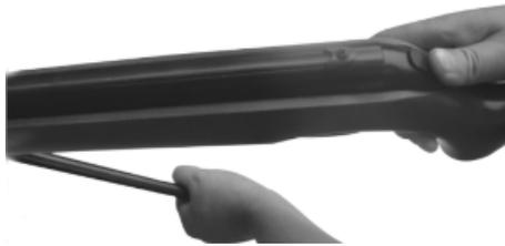
Fig.4 To return the underlever to its original position, first pull the underlever safety-catch located behind the trigger backwards. This will allow the underlever to be closed.
