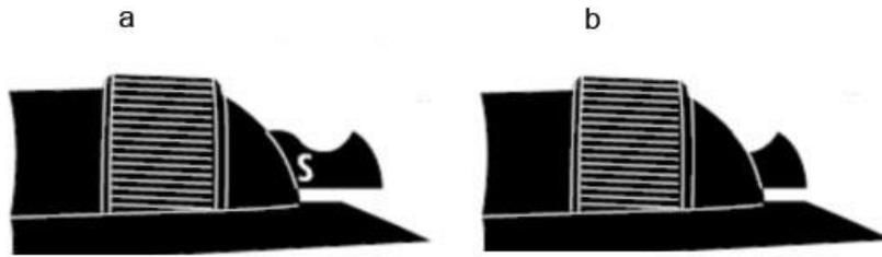
a : SAFETY “ON” ( ‘ S ’ is showing )    b: SAFETY “OFF” ( ‘ S ’ is not showing )
