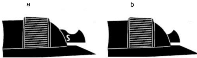
a : SAFETY “ON” ( ‘ S ’ is showing ) b: SAFETY “OFF” ( ‘ S ’ is not showing )
